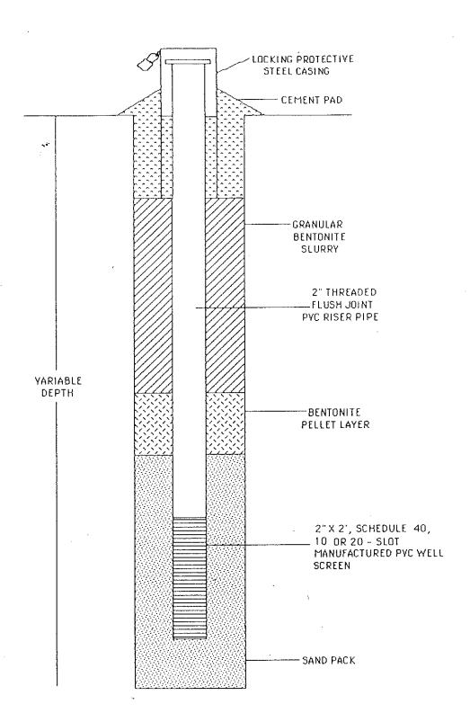
FIGURE 2-3 PROPOSED MONITOR WELL CONSTRUCTION SITE NO. 25 HIGGANAUM CONNECTICUT DEPT. OF TRANSPORTATION HAZARDOUS WASTE DISPOSAL SITE INVESTIGATION
