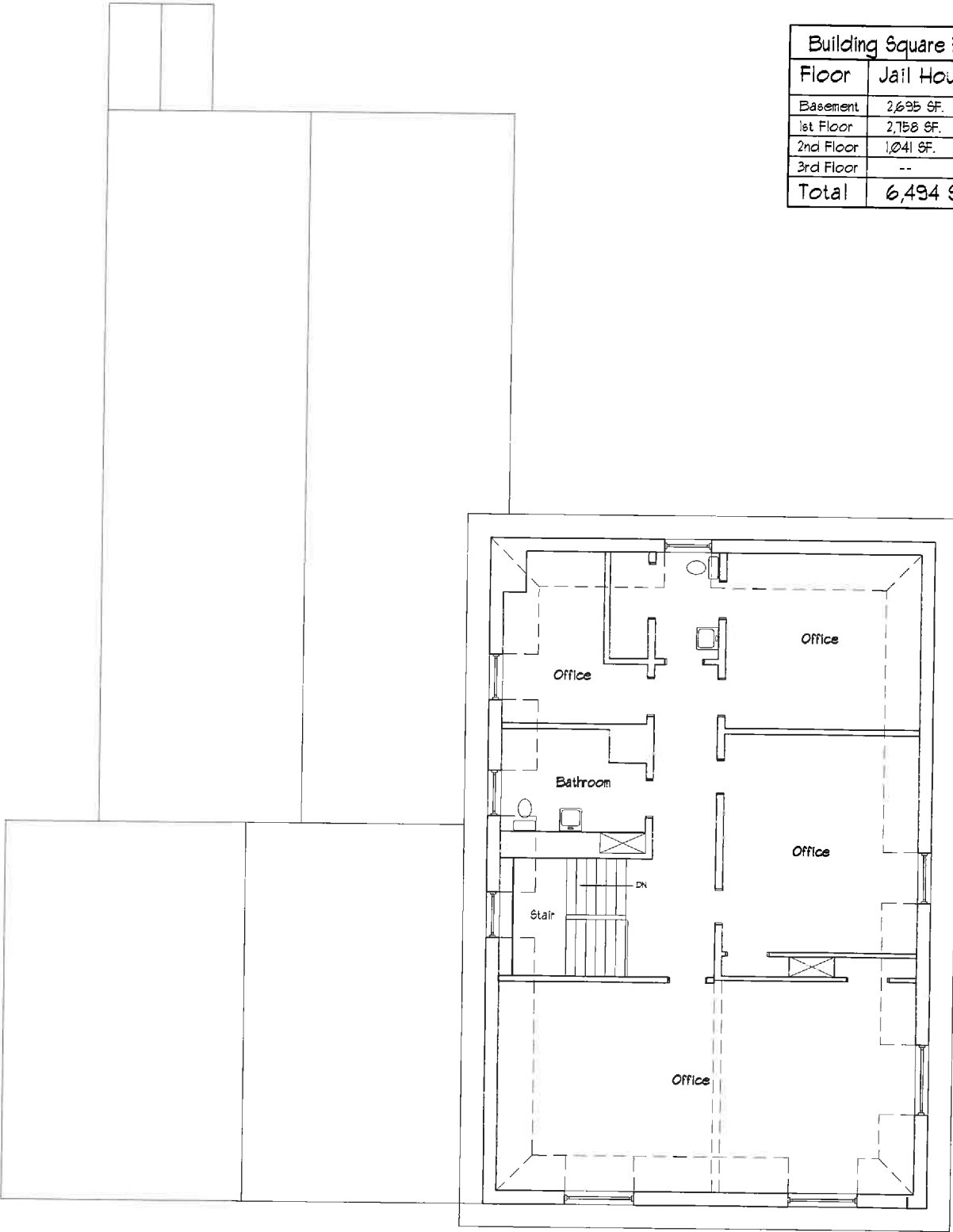
① THIRD FLOOR PLAN SCALE: 1/4" = 1'-0"
