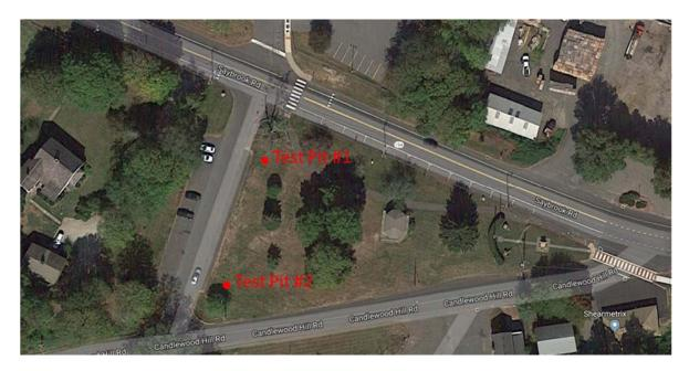
Two test pits were excavated at the Town Green on February 16, 2018 to determine the site suitability for wastewater disposal. Both test pits were located just east of the parking area and were found to have highly suitable soils for a subsurface sewage disposal system. Test Pit 1 (TP-1) was located at the
