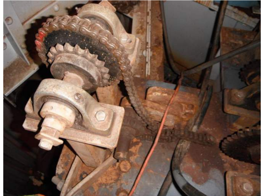
Photo M52: View of west auxiliary drive chain and sprocket attachment. Note light to moderate surface corrosion throughout the components and less than optimal storage conditions for the chain.
