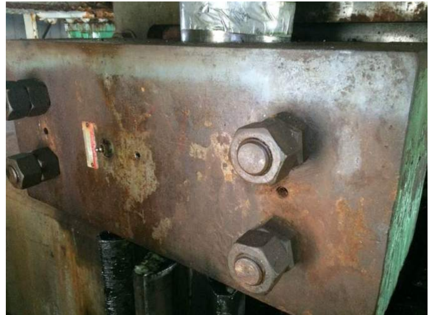
Photo M14: View of east lower pinion shaft bearing. Note three open holes in face.
