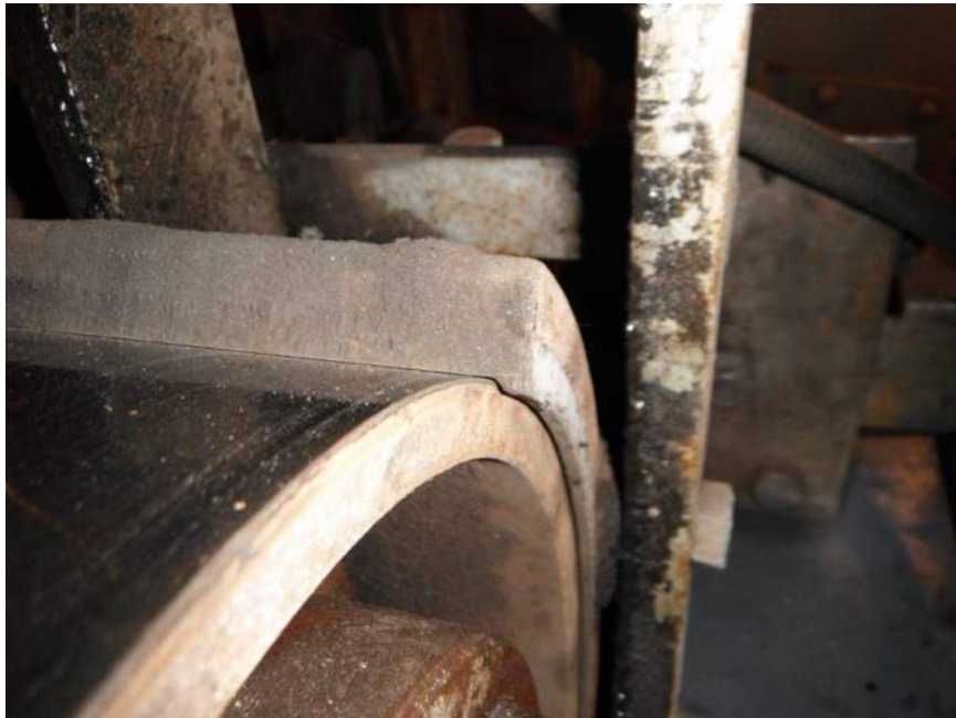
Photo M07: View of west machinery brake lining overhanging the brake wheel.
