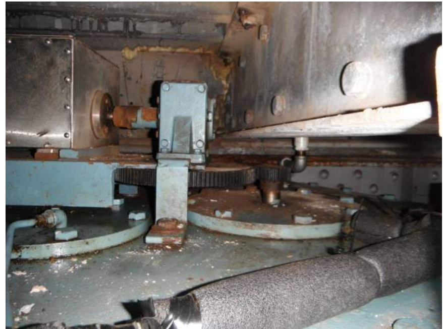
Photo M18: View of east span drive rotary cam limit switch drivetrain on top of the enclosed speed reducer. Note lack of corrosion protection on open gears.
