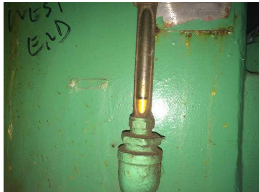
Photo M40: View west end wedge reducer oil level sight glass. Note oil level below that recommended by the manufacturer.
