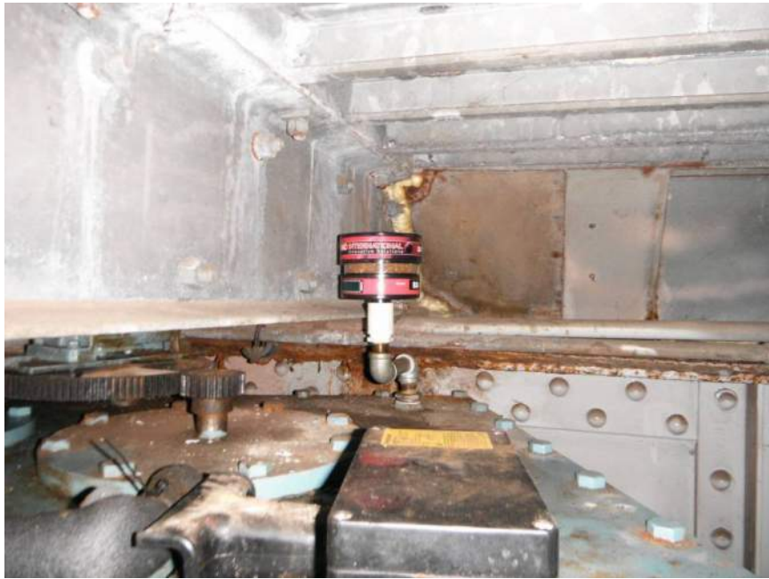
Photo M17: View of east span drive reducer desiccant breather requiring replacement.
