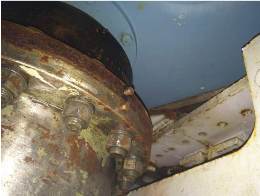
Photo M09: Close-up of purge plugs on west main pinion shaft coupling – plugs show signs of recent movement from maintenance activities.
