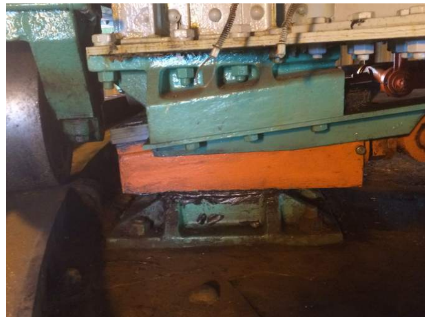
Photo M34: Corrosion on mounting bolts at SE wedge.
