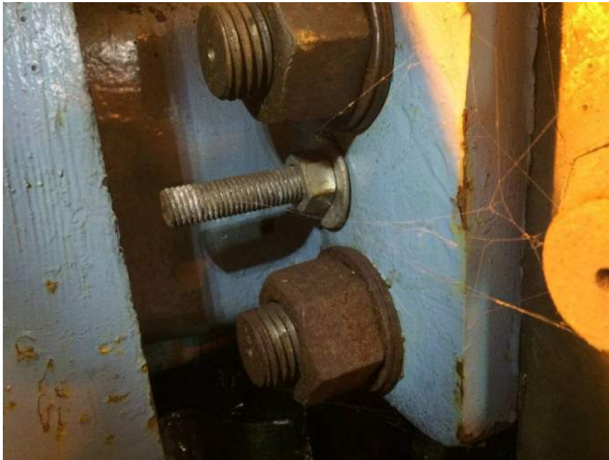
Photo M15: Note additional mounting bolt, likely from prior repair or replacement work.
