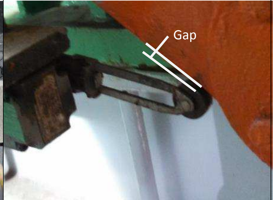
Photo E4 East Side Wedge Limit Switch Note that the switch arm is not making contact with the axel. .
