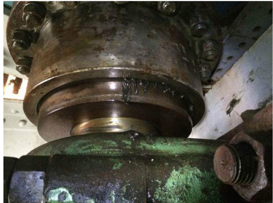
Photo M08: View looking up at lower half of west main pinion shaft coupling. Note grease actively purging from lower hub seal as noted during past inspections.
