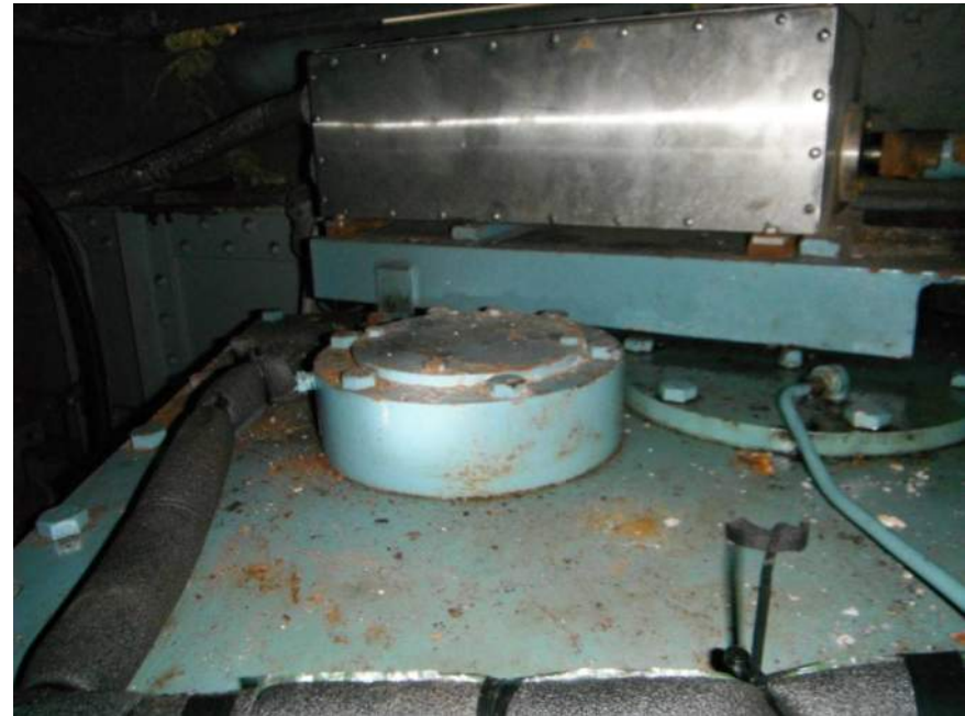
Photo M16: View of east span drive enclosed speed reducer. Note debris accumulation and surface corrosion on top of unit.
