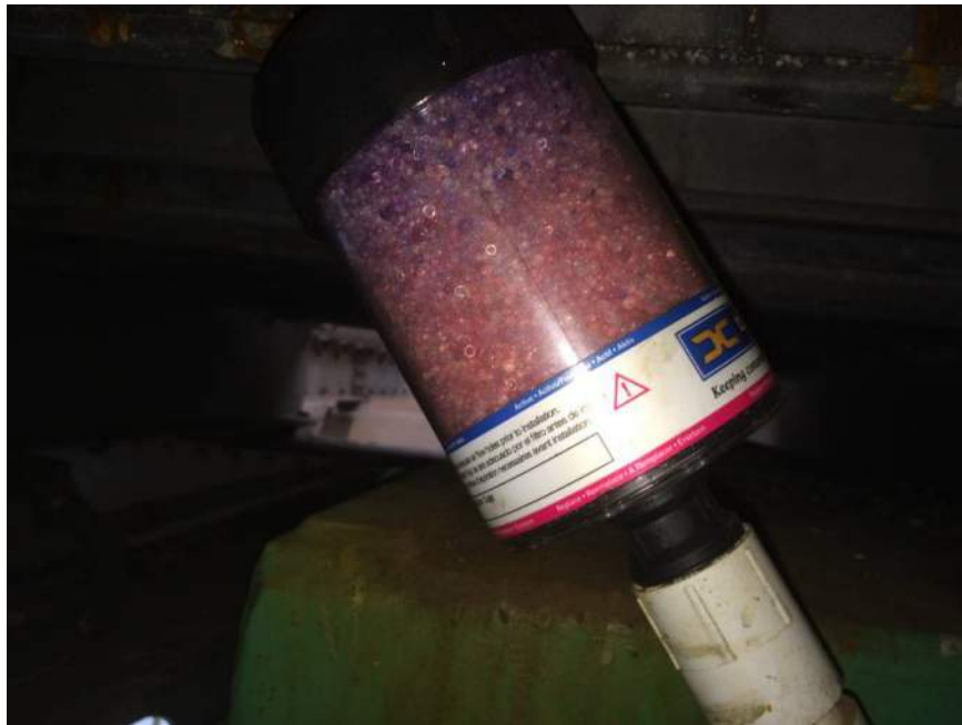
Photo M41: View of west end wedge gear reducer desiccant breather. Note almost all desiccant has changed color to pink, indicating the breather requires replacement.
