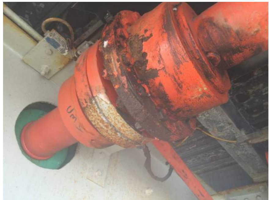
Photo M42: View of west end wedge C2 single engagement gear coupling. Note moderate paint failure and surface corrosion.
