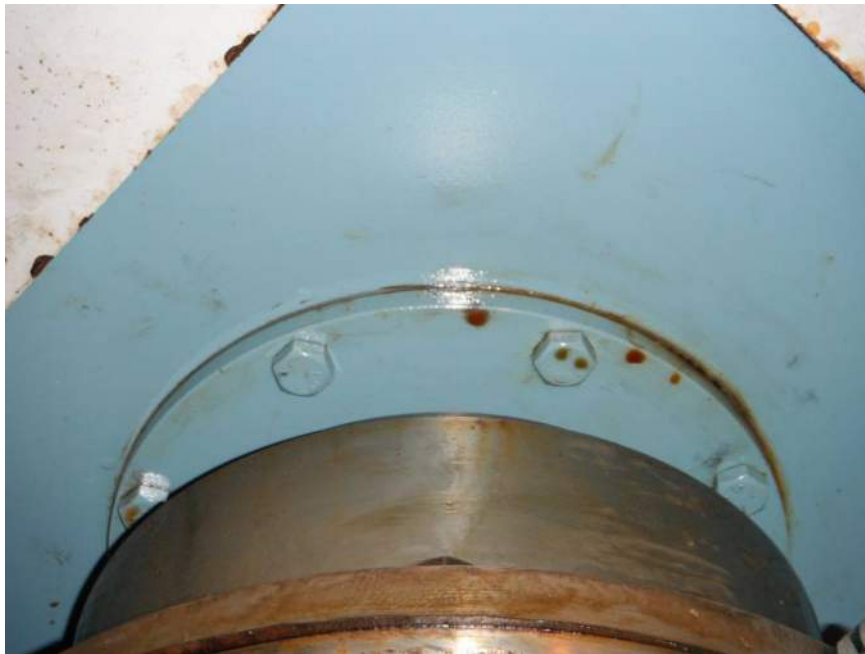
Photo M19: View of possible light oil seepage from east enclosed speed reducer output shaft bearing.
