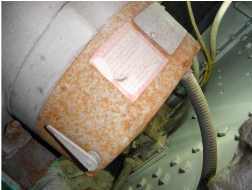
Photo M37: View of north center wedge brakemotor housing. Note lack of paint protection and developing surface corrosion.
