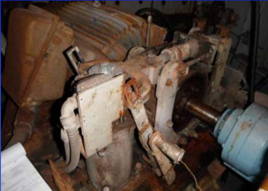
East Machinery Brake Manual Lever No Longer Locks
