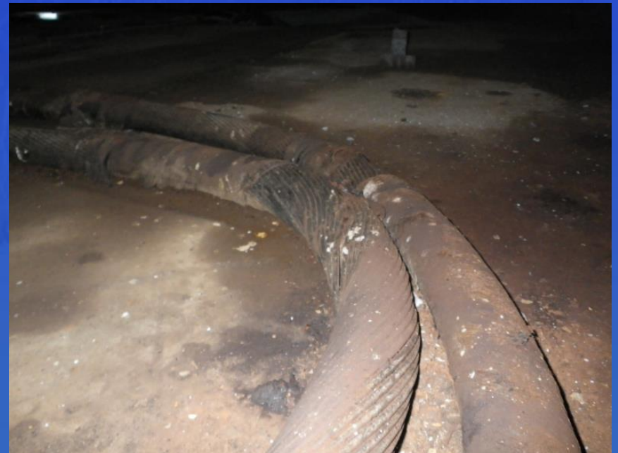
Submarine Cables Missing Protective Jacket
