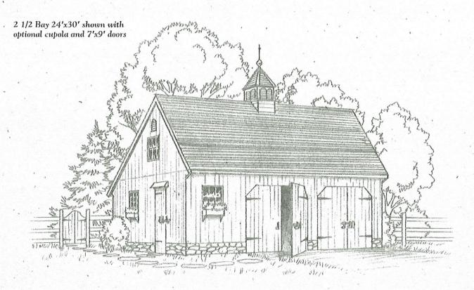
In addition to an added two feet of space front to rear, our top of the line 24' Saltbox Carriage House has a third beam and a center post built into the kit which allows for a loft. Both our 22' and 24' Saltbox models have the genuine look and feel of old-time carriage houses.
